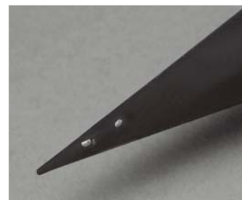
Fig. 3 Eroded tip of the projectile after tests.
